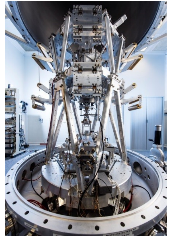
Kibble balance (to measured Planck constant h )
