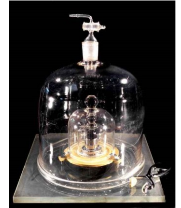
IPK - international prototype of the kilogram (platinum-iridium alloy)
